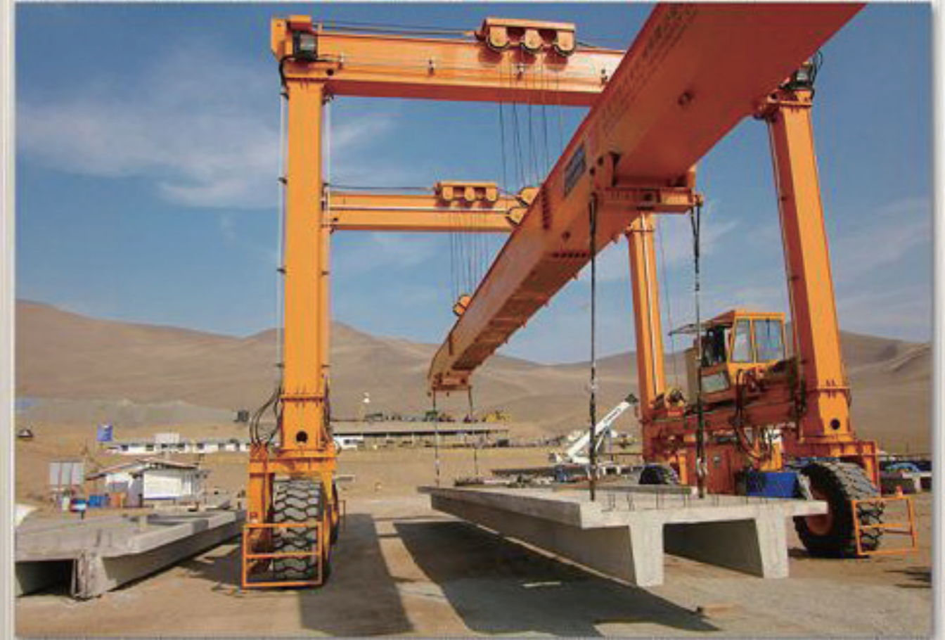
Straddle Carrier (50 ton capacity) TITAN, Peru
