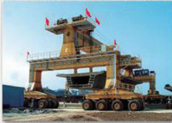
Gantry Special Carrier / 3rd BG CRCC
