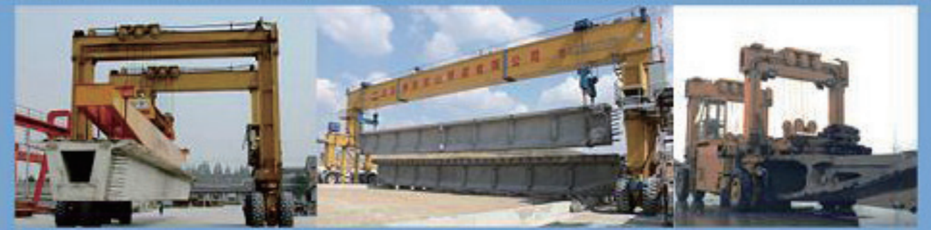
Straddle Carrier/Mobilift(180 ton capacity)/SCG
