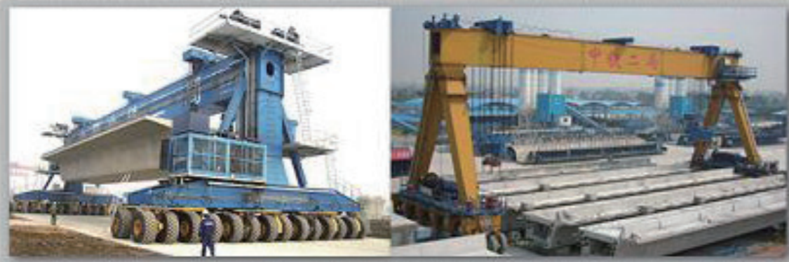
Special Carrier (300 ton capacity) for Harbin-Dalian Highspeed Railway / 2nd BG CREC
